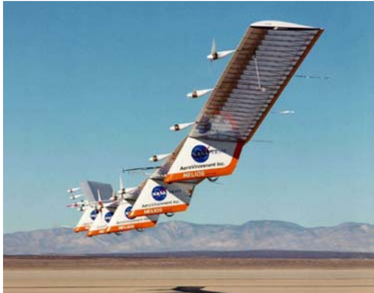
The Heleos solar-electric airplane, by AeroVironment and NASA, capable of continuous flight for 6 months at 20,000 meters.
